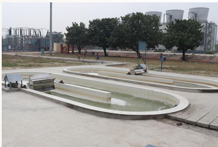
Figure 10. CO 2 capturing using microalgae at Pata. Credits: GAIL.
