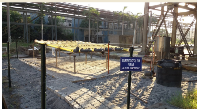
Image 12 Photo bioreactor of 1000 litres capacity
